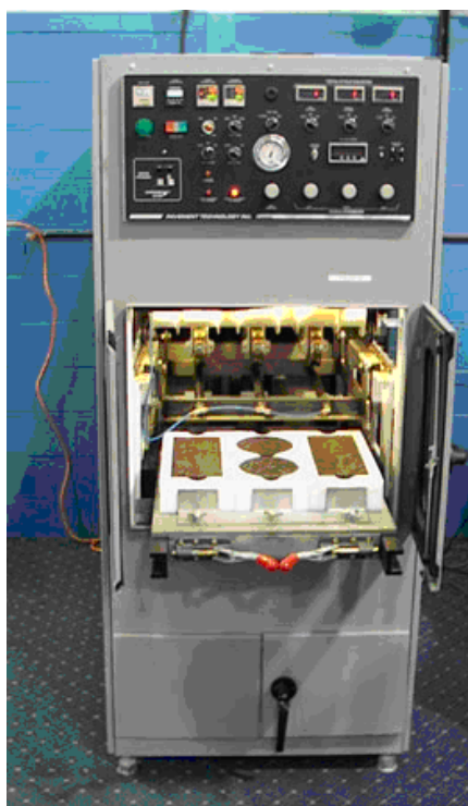
Figura 169 - Asphalt Pavement Analyzer -APA - http://pavementinteractive.org/
