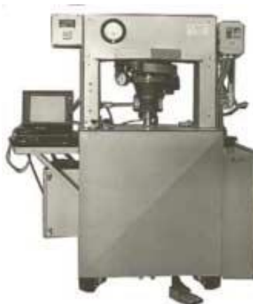
Figura 135 - Compactador Giratório Texas (op. manual) http://www.tfhr.gov/pavement/asphalt/labs/mixtures
