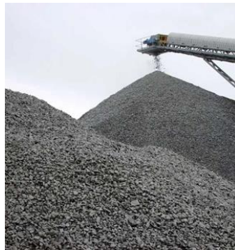
Figura 5 - Brita 1", \frac{1}{2} ", pedrisco, pó de pedra, etc.
